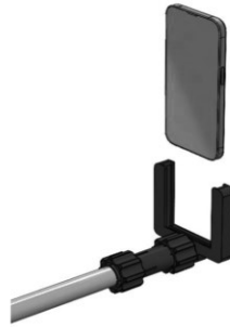
Inserting smartphone into mount and launching app
